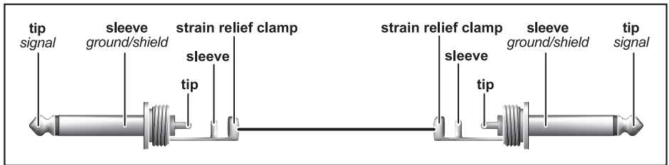
Fig. 4.1: Patch cord with unbalanced, 1/4" TS plugs
